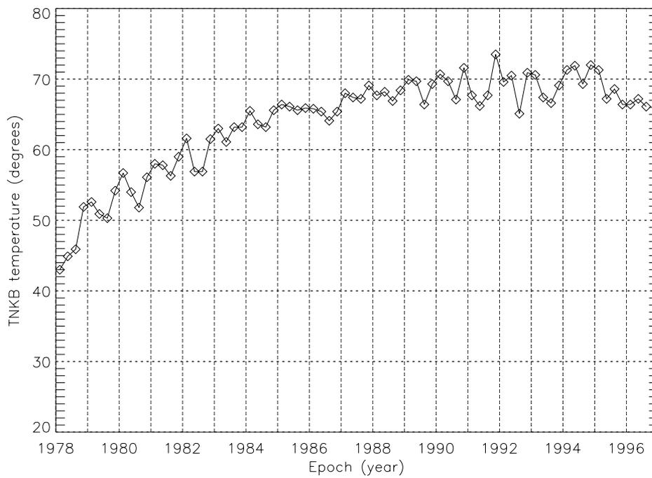
Figure 6-6. History of average hydrazine tank B temperatures.
