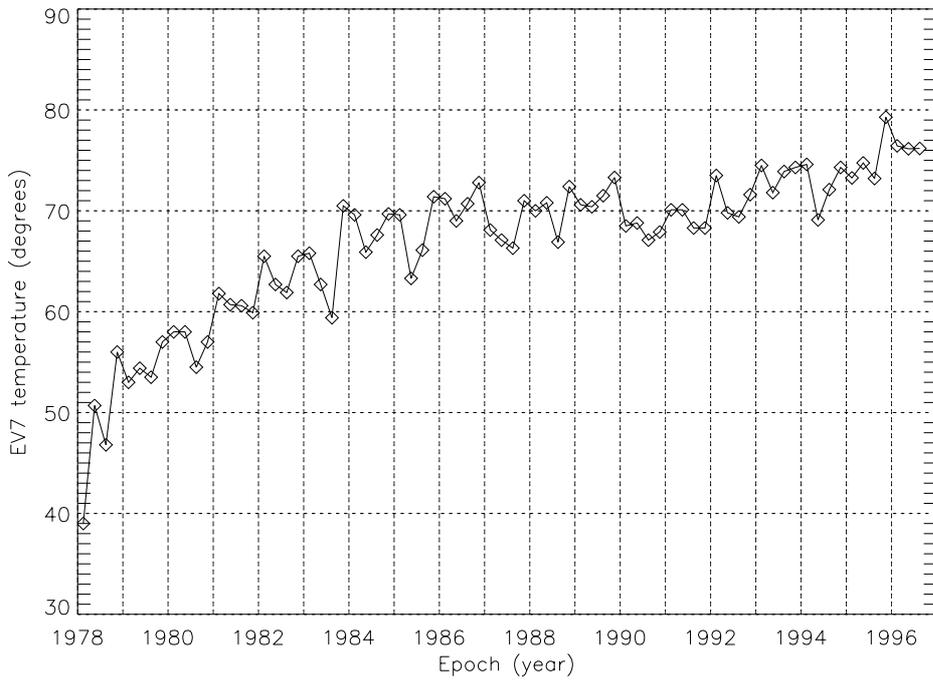
Figure 6-9. History of average engine valve 7 temperatures.
