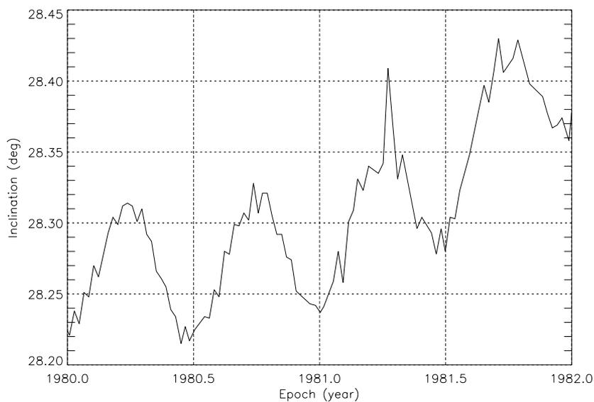
*Figure 4-10. Periodical changes in inclination.*
