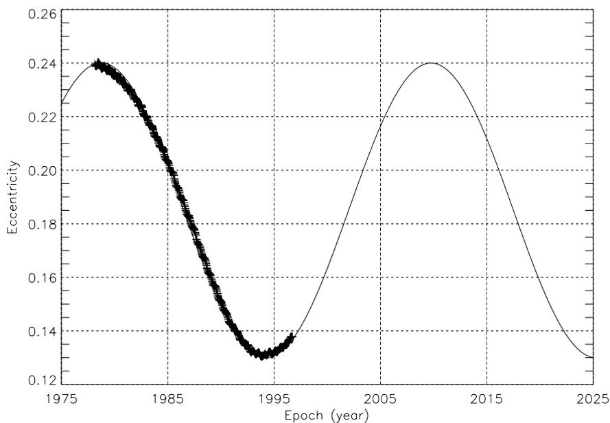
*Figure 4-7. Predicted Long-Term Changes in IUE Orbital Eccentricity.*
